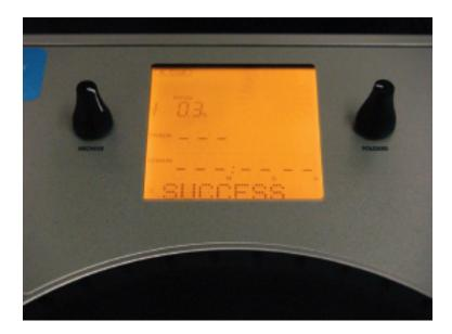
During the update the unit will flash Update and Success twice if the firm ware has been updated correctly. In some cases you may get a Failure display if this does happen please wait until the process if completely finished and the disc to eject. Then simply power the unit off then on again and repeat the update steps.
